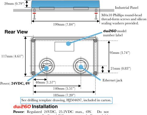
connect to a distributed DC power network. External 1A fast-acting fuse or 1A current-limiting is required!
